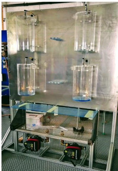
Figure 2: Pilot scale four tanks system.
