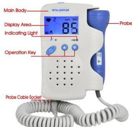
**Figure 2-6:** *Fetal Doppler heart sound monitor device displaying fetal heart rate [39].*
