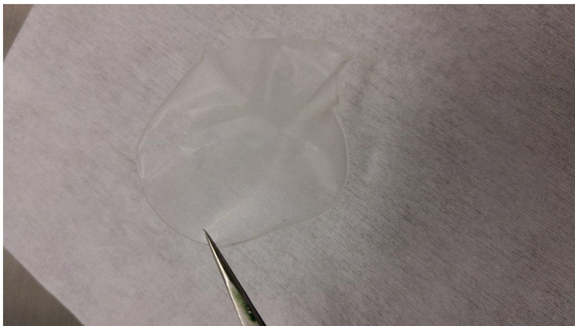
Figure 21: Image of the pure PVDF-HFP (Transparent) polymer film.
