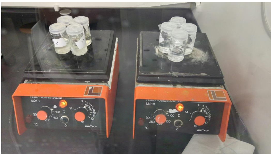
Figure 30: Preparation of different electrolyte films in magnetic hot plate.
