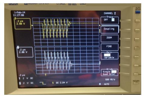
Figure 33: The output from CPLD for 8 pulse cycle.
