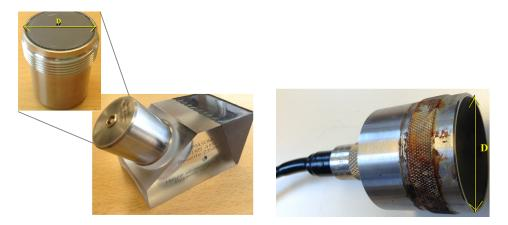
Figure 18: Single element ultrasound transducers.
