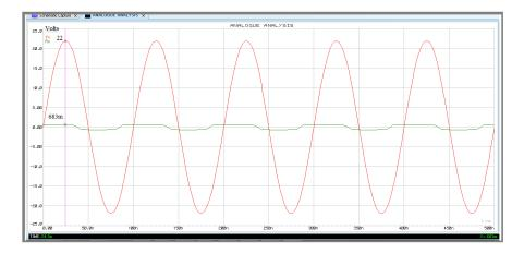
Figure 38: The simulation of T/R switch in Protetus.
