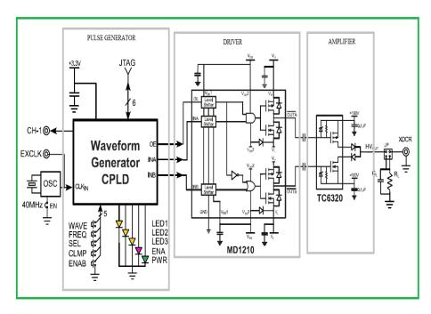
Figure 8: The MD1210DB transmitter board circuit diagram [1].
