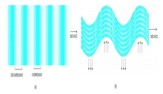
Figure 1: Sound wave propagation; Longitudinal wave (Left), Transverse wave (Right).
