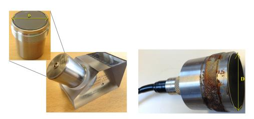
Figure 3: Single element ultrasound transducers.
