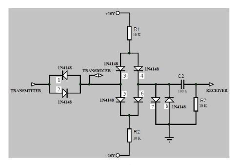
Figure 11: A single channel T/R switch passive circuit.
