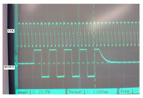
Figure 34: The AC coupled local oscillation output (top) from PCB4(Figure 6) and the HVOUT (bottom) from PCB1(Figure 6).
