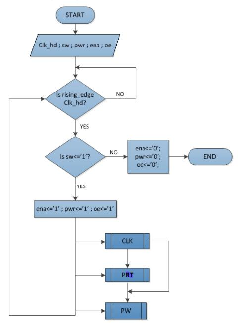
Figure 25: The flow char of the top level process MAIN in the design.
