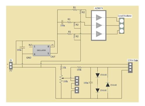
Figure 15: The oscillator and gain board circuit diagram.
