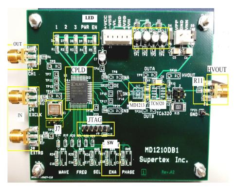
Figure 7: The MD1210DB transmitter board [1].
