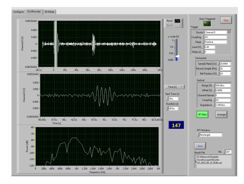
Figure 35: Ultrasound investigation using 1 MHz single element transducer in water.
