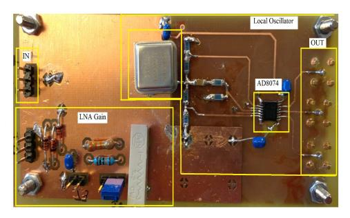
Figure 14: The oscillator and gain board.
