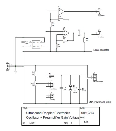
Figure 37: Oscillator and gain board reference circuit [4]
