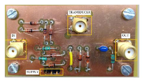
Figure 10: A single channel T/R switch PCB.
