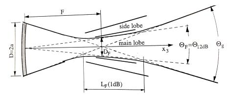
Figure 4: Ultrasound beam focusing from spherical shell disc (D is aperture, a is wavelength of the ultrasound) [5].
