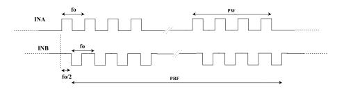
Figure 9: The outputs INA and INB from the CPLD.
