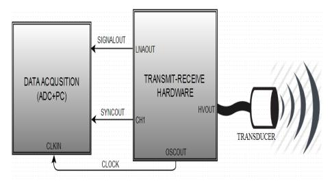
Figure 5: The overall system block diagram.
