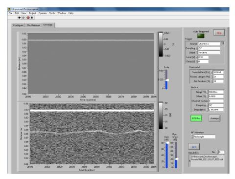
Figure 36: M-mode ultrasound investigation for 1 MHz single element transducer in water.
