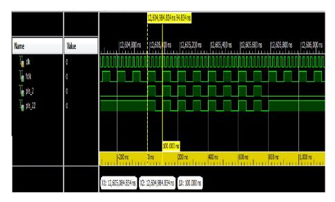
Figure 31: The behaviour simulation of the beamformer for the eigh pulse cycle.
