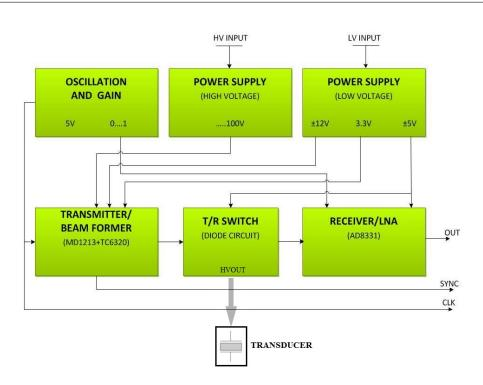
Figure 6: The ultrasound transmit-receive system block diagram .
