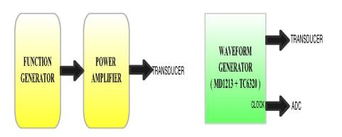
Figure 2: Block diagram of conventional analog function generator (left) and the digital waveform generator (right).
