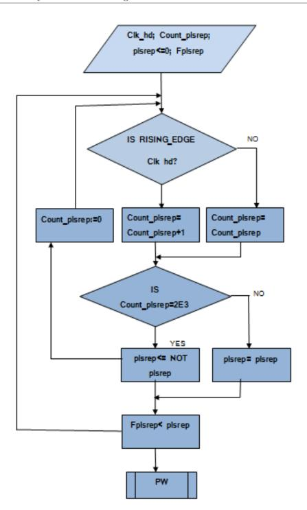
Figure 27: The flow chart for pulse repetition rate PRT module in the design.
