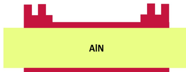
Figure 4.10. Schematic of the FBAR with two pairs of acoustic mirrors
