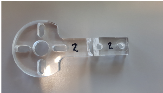
Figur 5.21: Brudd over innspenningshull
