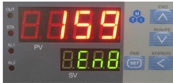
Fig. 2.6 Temperature controller panel
