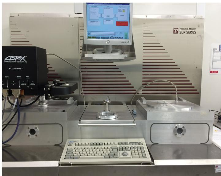
Fig. 2.9 Reactive Ion Etcher
