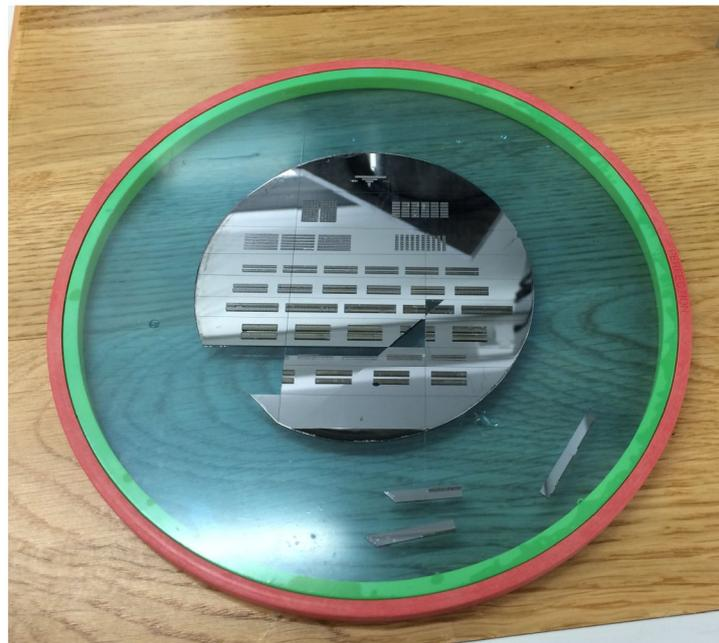
Fig. 5.6 wafer after finishing SU-8 process
