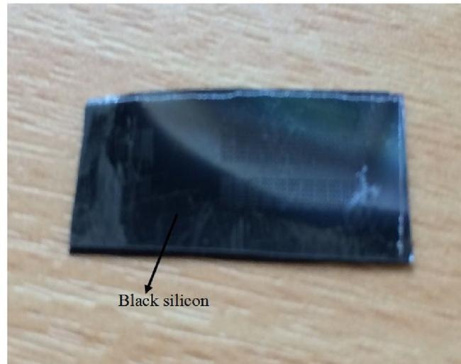
Fig.4.6 wafer 1 RIE etching for 15mins
