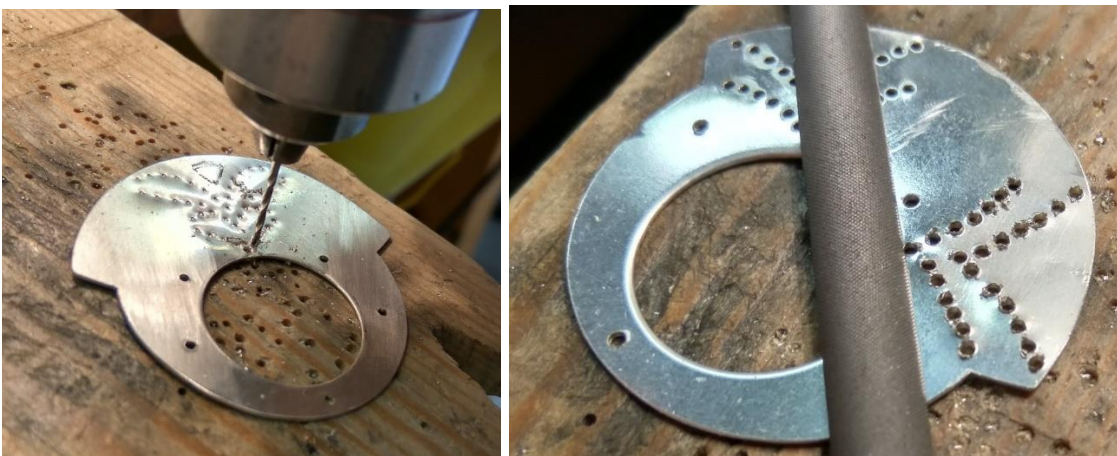
Fig. A4-29 The process of drilling with a 1mm drill bit
