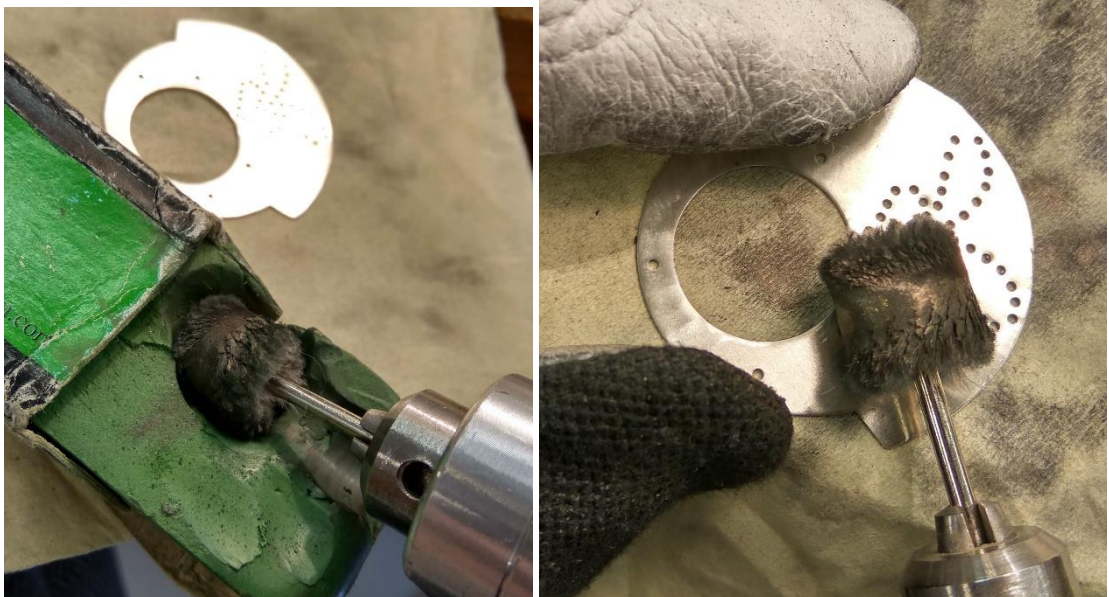
Fig. A4-32, 33 The process of polishing the silver
