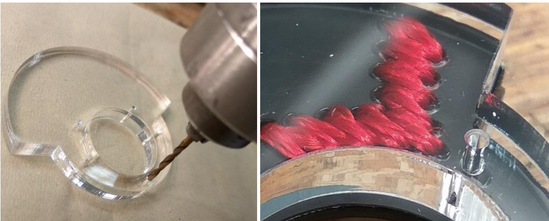
Fig. A4-14 The process of making the hole bigger with a flexible shaft machine
