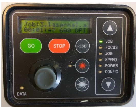
Fig. A4-2 The display with function menu on the laser-cutting machine
