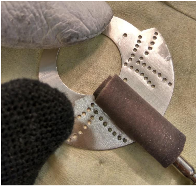
Fig. A4-31 The sandpaper processing with the flexible shaft machine
