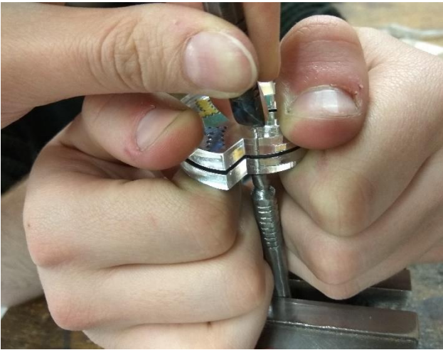
Fig. A4-20, 21 The process of forming the rivet head
