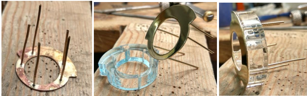
Fig. 96-98 The process of making the ring with one acrylic part and one metal part
