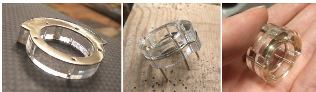
Fig. 93-95 The process of making the ring with two acrylic parts and one metal part between
