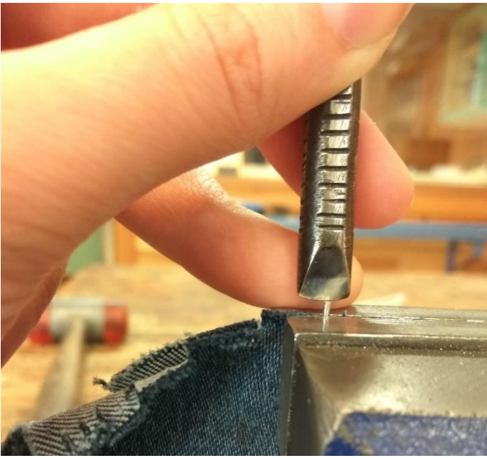
Fig. A4-13 The process of making the “head” of the rivet
