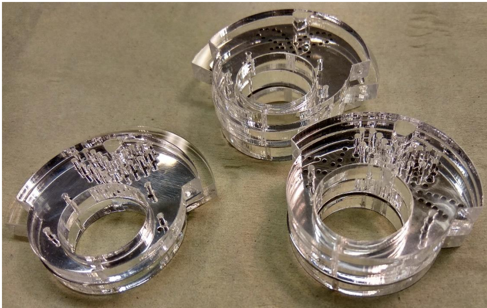
Fig. 132 The layers of acrylic and silver in the right order
