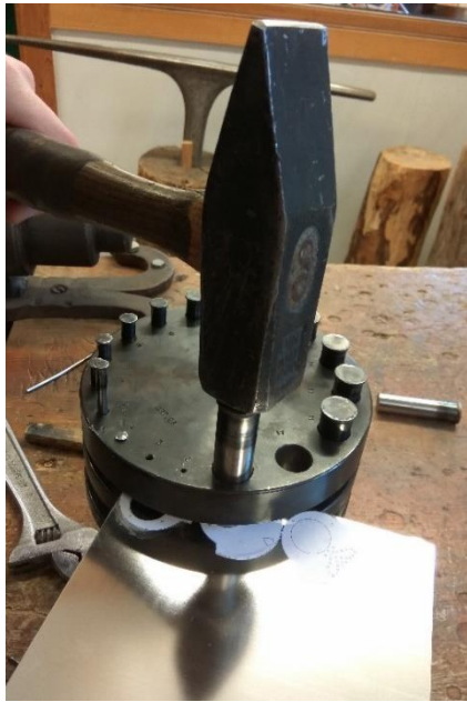
Fig. A4-23 The process of the punching
