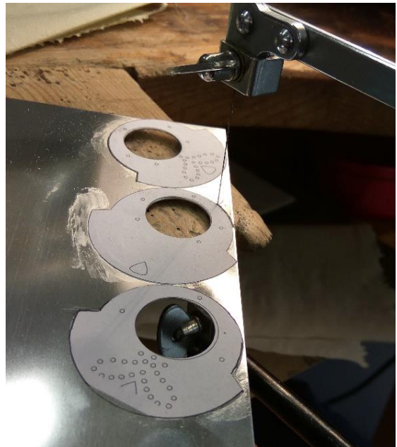
Fig. A4-24 The process of the cutting out the silver parts
