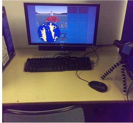
*Figure 9.* Workstation of the Master equipped with a RADAR, visual lookout, a keyboard and a mouse.
