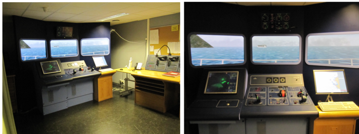
Figure 3. The ship simulator Frøya with a control panel, map table, radio and LCD displays.
