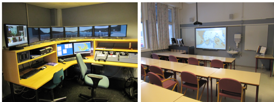
Figure 4. On the left, the instructors' control room is shown. Here, the instructors guide the exercises and communicate with the five simulators. On the right, the brief/debrief room is shown; it has a smart board that enables trainers to replay the exercises.
