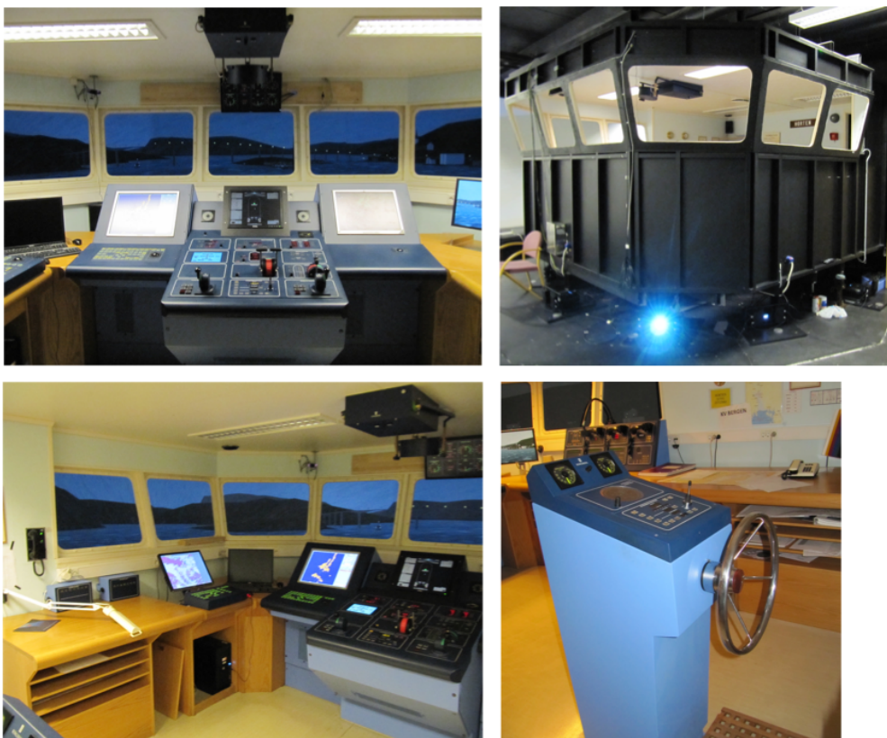
Figure 2. The full-mission ship simulator Bergen: the main control panel with thruster controllers, the exterior of the bridge replica with projectors underneath it, the map table and the steering wheel.
