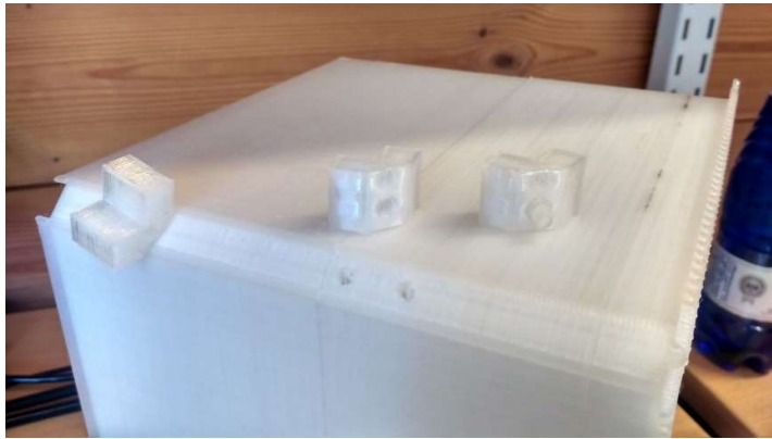
Figure 61: Experiments with the connection (attempt at printing a full scale object)
