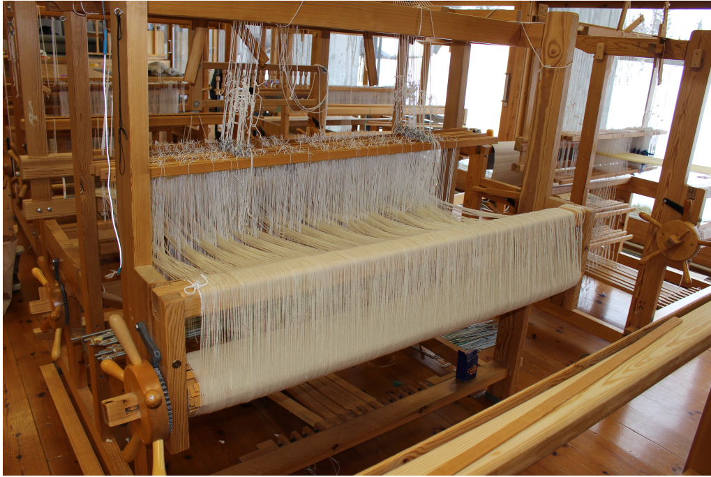
Fig. 40 The shaft draw system that I prepared for weaving the blankets, photographer Heidit Vares
