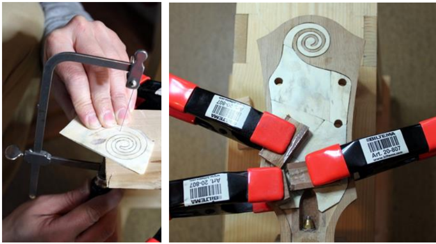
Figure 70 Cutting and Gluing Headstock Antler Plates
