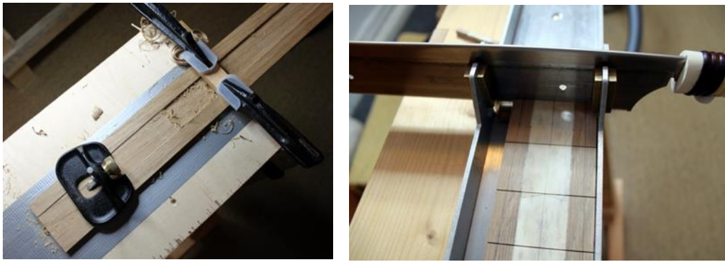
Figure 72 Routing for the Neck Inlay and Cutting the Frets Slots
