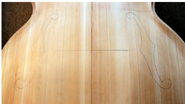
Figure 57 "F" Holes Position in the Top Plate
