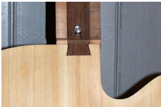
Figure 63 Neck and Body Joint
