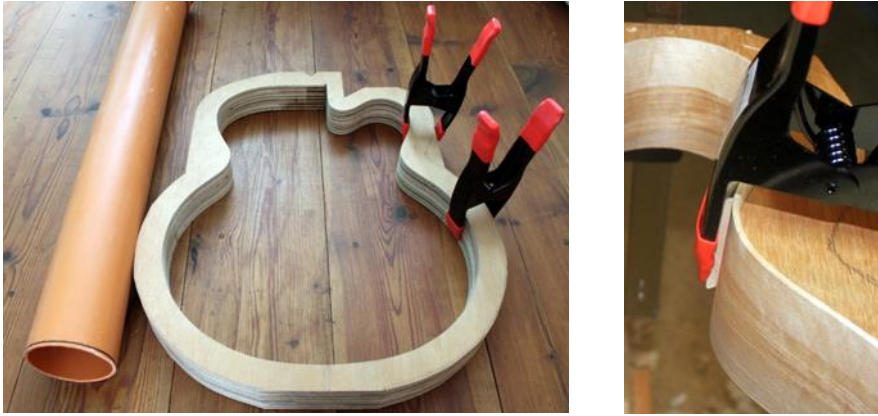
Figure 58 Bending the Sides
