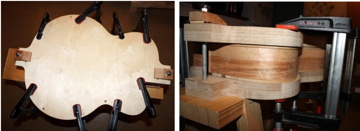
Figure 61 Gluing of the Top and Back Plates
