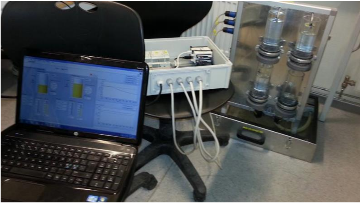
Figure 2-1: Real 4-Tank system connected to the computer system
