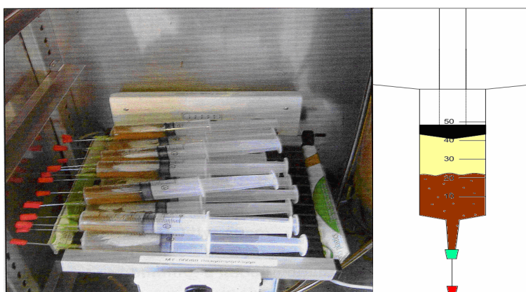
Figure 2.1 Batch experimental setup. The left figure shows the overview of batch experiment setup with syringes on a shaker in an incubator; the right one shows a single syringe as an anaerobic digester with a rubber stopper.
