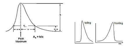
Figure 3-12: A sketch of peak asymmetry, tailing and fronting.[31]
