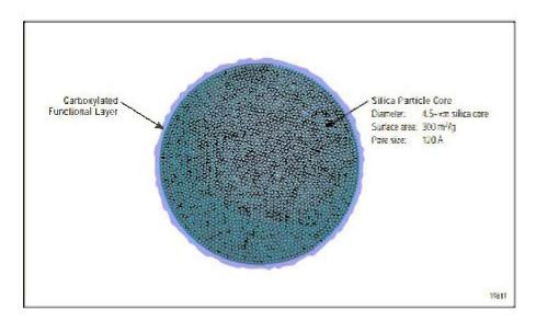
Figure 4-2: Structure of the IonPac SCS 1 Silica Cation Separator packing particle.[33]
