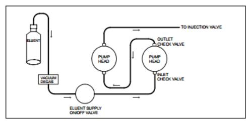
Figure 4-4: Isocratic Pump Flow Schematic.[35]
