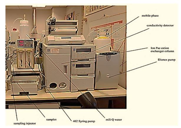
Figure 4-1: The cation chromatograph apparatus.
