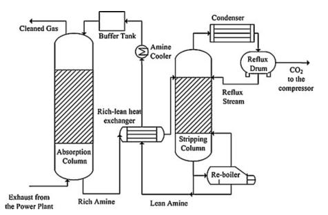
Figure 2-9: Flow sheet for CO<sub>2</sub> capture from flue gases using amine-based system.[13]
