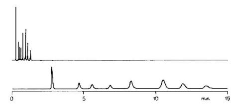
Figure 6-6: Above) 6cm x 4.6 mm i.d column with 3µm material. Below 20cm x 4.6 mm i.d column with 10µm material.[46]
