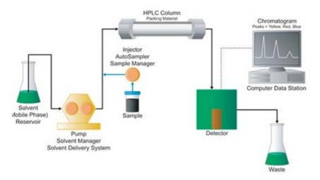
Figure 3-3: General design of a system for ion-exchange chromatography. [20]
