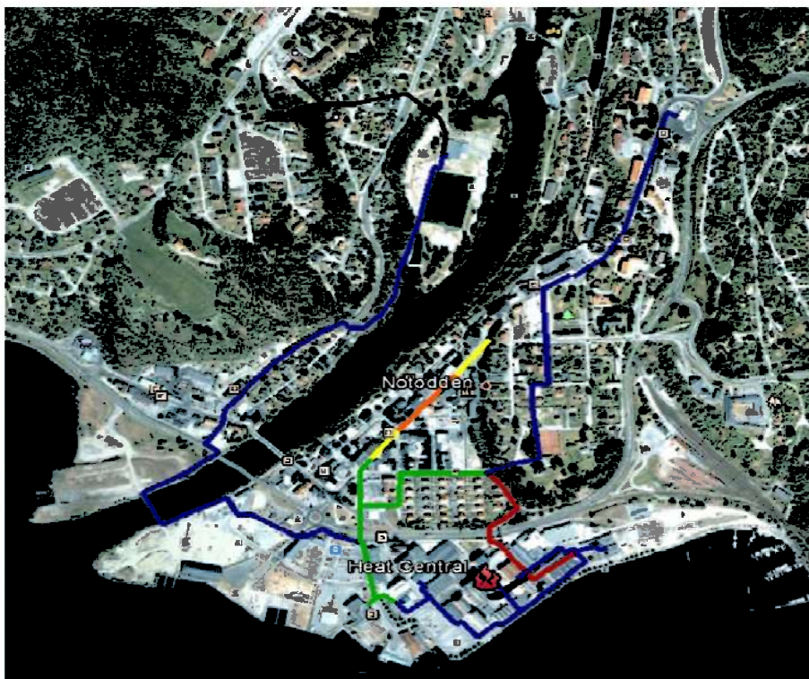
Figure 3-1 Notodden district heating system distribution piping (Google Earth, 2012). Yellow – DN80, Orange – DN100, Green /Black – DN125, Blue – DN150, Red – DN200
