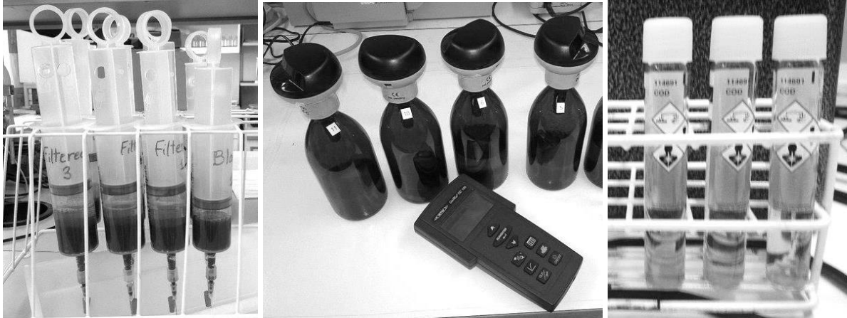
Figure K-2 : Main step of biogas potential test, BOD and COD measurements
