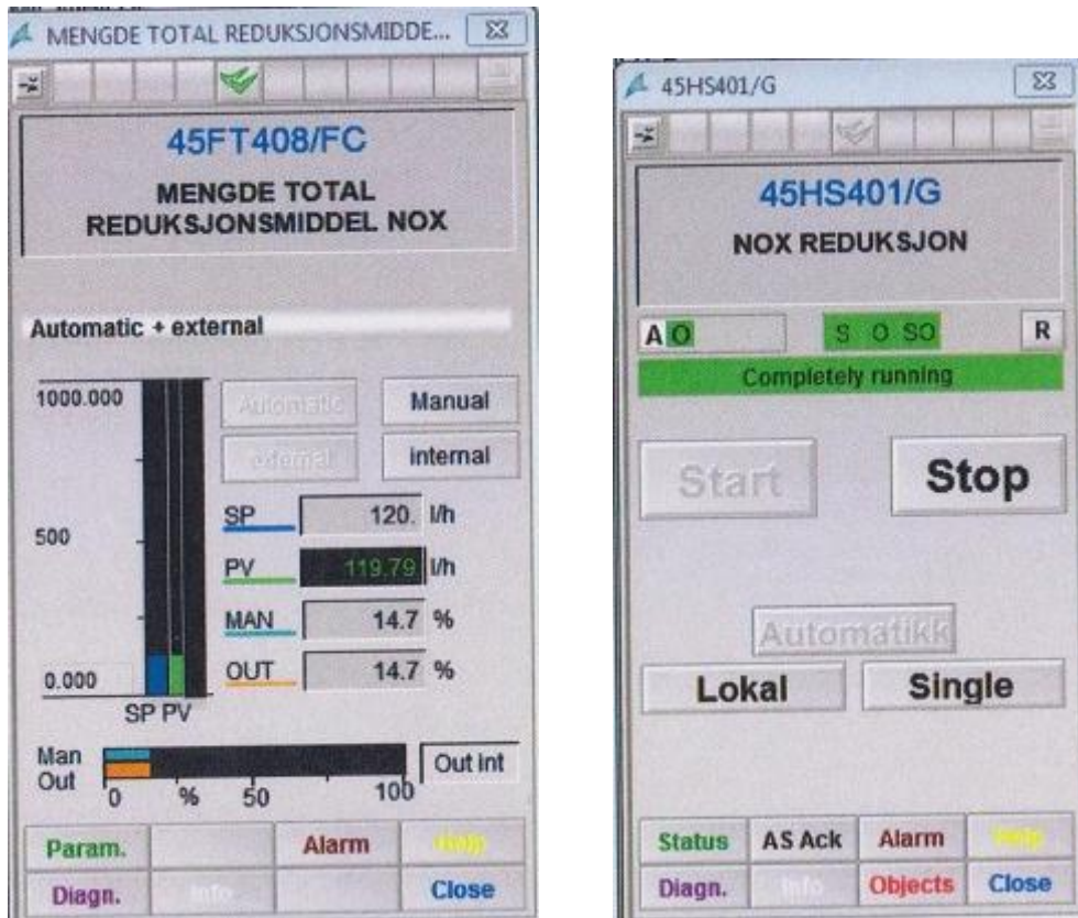
Figure 5-1 NOx reduction system regulators
