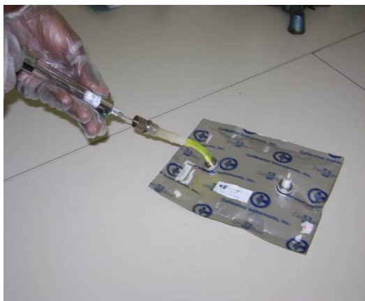
Figure 5.20: Gas taking from gas bags
