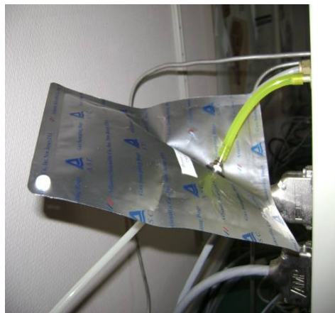
Figure 5.19: Exhaust collect in gas bags
