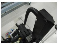
Figure 3-5 Fiber optical slit connected to the halogen lamp.
