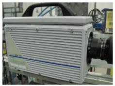
Figure 3-3 High-speed camera.
