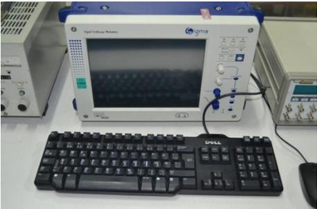
*Figure 3-9 Sigma Oscilloscope.*
