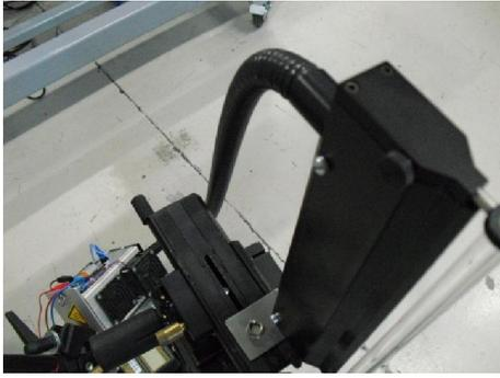
*Figure 3-5 Fiber optical slit connected to the halogen lamp.*
