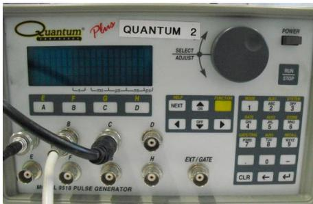
*Figure 3-7 The pulse generator.*
