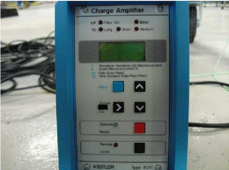
*Figure 3-8 The amplifiers for the pressure sensors.*
