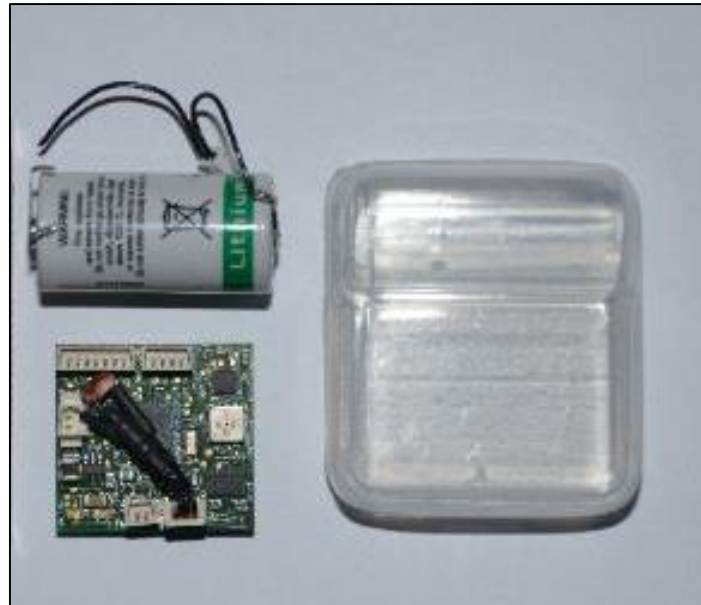
Fig. 4. Tri-axial acceleration data logger (27x26x8 mm, 20g) with the battery and casing developed by Swansea University.
