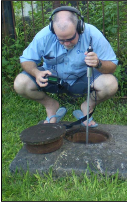
Figure 17: Listening stick (left) and Geophones (right) (Source: Author, 2006)
