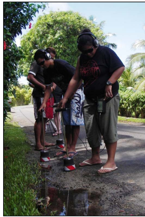
Figure 17: Listening stick (left) and Geophones (right) (Source: Author, 2006)
