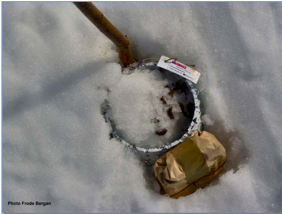
Fig. 3 The collection of faecal pellets from each roost was arranged in a 20 cm long and 15 cm diameter piece of pvc pipe, perforated and painted white to eliminate overheating. A temperature logger wrapped in beige-colored paper was situated adjacent to the pipe in order to record when the collection of pellets emerged at the snow surface (indicated by alternating day/night temperature) during the spring snow melt (photo Frode Bergan).
