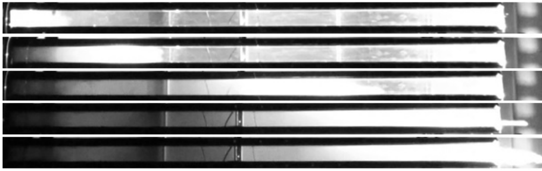
Figure 5. Photo of carbon dioxide propagation with the 1.0 mm nozzle
