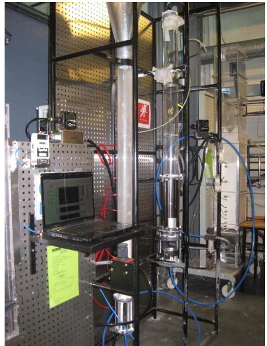
Fig. 1: Experimental set-up. Fluidized bed with pressure reduction valve, digital flow controller, pressure sensors.
