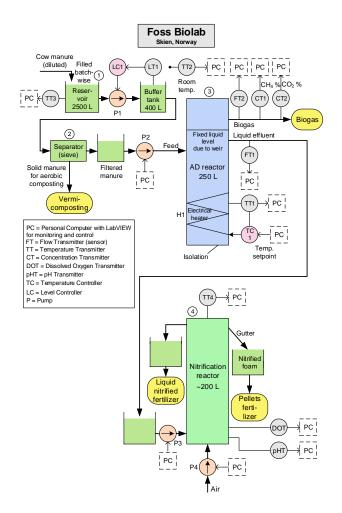
Figure 1: Piping & Instrumentation Diagram (P&ID) of the biological process line of the pilot plant at Foss Biolab, Skien, Norway. This paper concerns the AD reactor.
