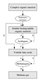
Figure 2: The anaerobic digestion steps forming the basis of Hill's model. The alphabetic indicators refer to Hill's model, eqs. (1)-(10). The symbols resemble those in Zaher et al. (2009).
