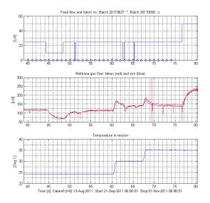
Figure 7: Reactor ADR1: Responses in  $F_{meth}$  (middle) due to changes in  $T_{reac}$  (lower) and  $F_{feed}$ (upper).
