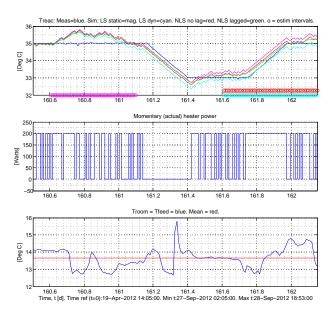
Figure 8: Upper plot: Real (measured) and simulated  $T_{reac}$ , and time intervals for estimation (marked 'o'). Middle plot: Real  $P_{heat}$ . Lower plot:  $T_{room} = T_{feed}$ .
