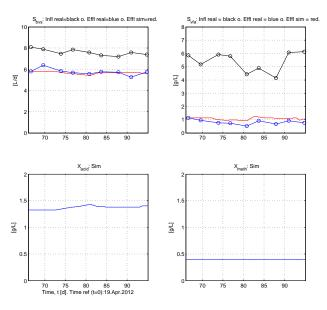
Figure 6: Upper plots: Real values (from laboratory analysis) and simulated values of the state variables  $S_{bvs}$  and  $S_{vfa}$  together with the respective real concentrations in the feed. Lower plots: Simulated values of the state variables  $X_{acid}$  and  $X_{meth}$  for which we do not have laboratory analysis data.
