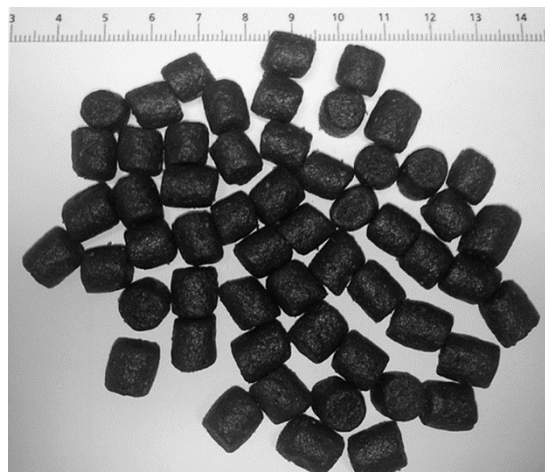
Figure 2: Fish feed pellets (Skretting, Optiline 2500) used in this study. Length = 10mm and diameter = 9mm.
