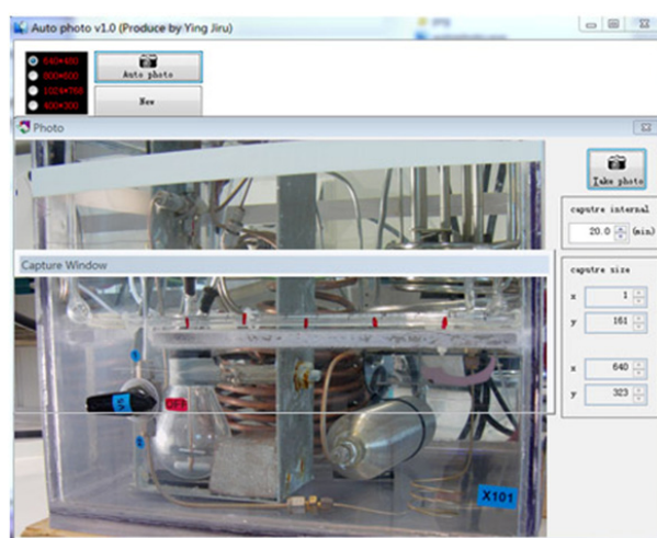
Figure 3.8 The interface of the sub-program “Auto Photo” for capturing the position of the mercury drop of the novel solubility measurement setup
