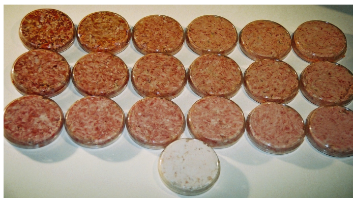
Figure 16. Petri-dishes with meat/fat mixtures. From top to bottom: Bovine, Bovine/Pork, Pork and pure fat. Fat content increases from left to right. Glass covers were removed just prior to imaging.
