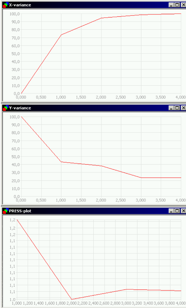
Figure 6. Calibrated X-variance (top) and Y-variance (middle) and validated PRESS (low) for the crispbread case in figure 2.
