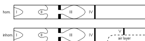
Figure 1: A sketch of the experimental setup, homogeneous on top and inhomogeneous below.
