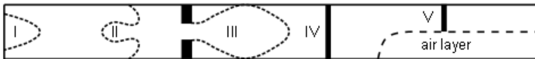
Figure 2.1: A sketch of the geometry with the different stages of combustion wave propagation from ignition and tulip flame to DDT and detonations in layers.
