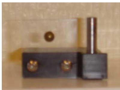
Figure 4-5. A known object. The diameter of the sphere is 4 mm. The diameter and height of the cylinder are 4 mm and 13 mm, respectively.
