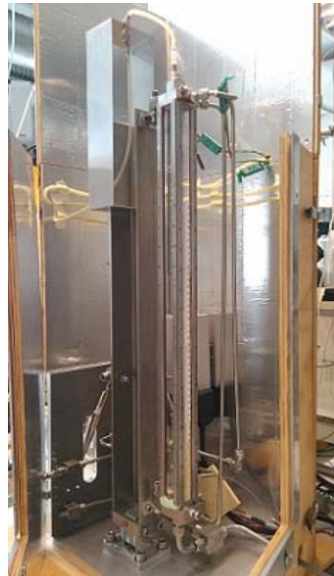
Figure 5-3. The picture of the novel experimental apparatus for studying gas absorption into liquid droplets.
