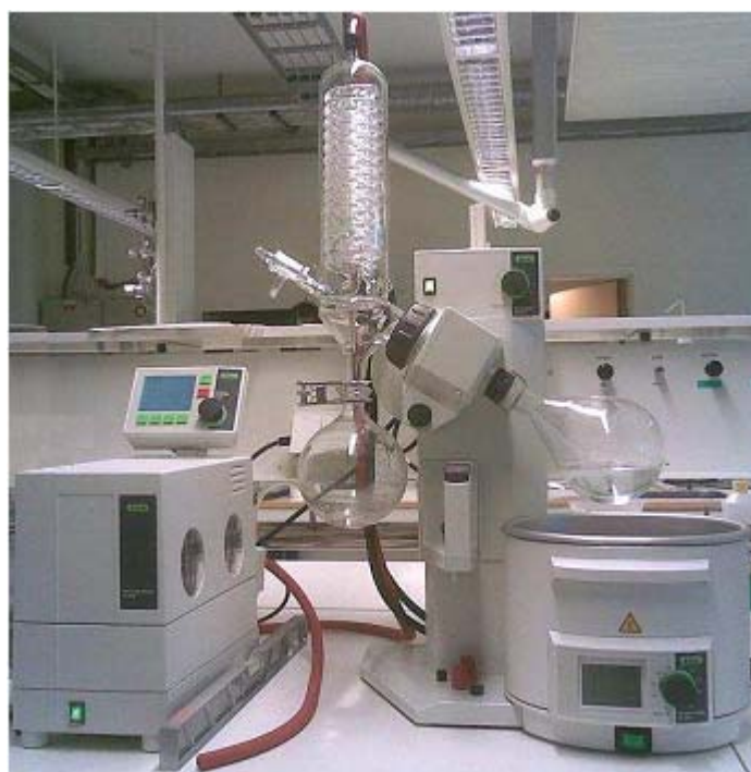
Figure 3-1. The rotary evaporator for degassing distilled water and pure amines.
