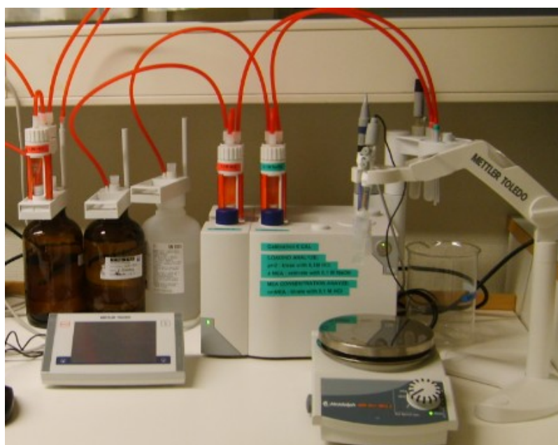
Figure 3-4. Titrator T50 used for analyzing the amount of CO 2 in the loaded amine solutions.
