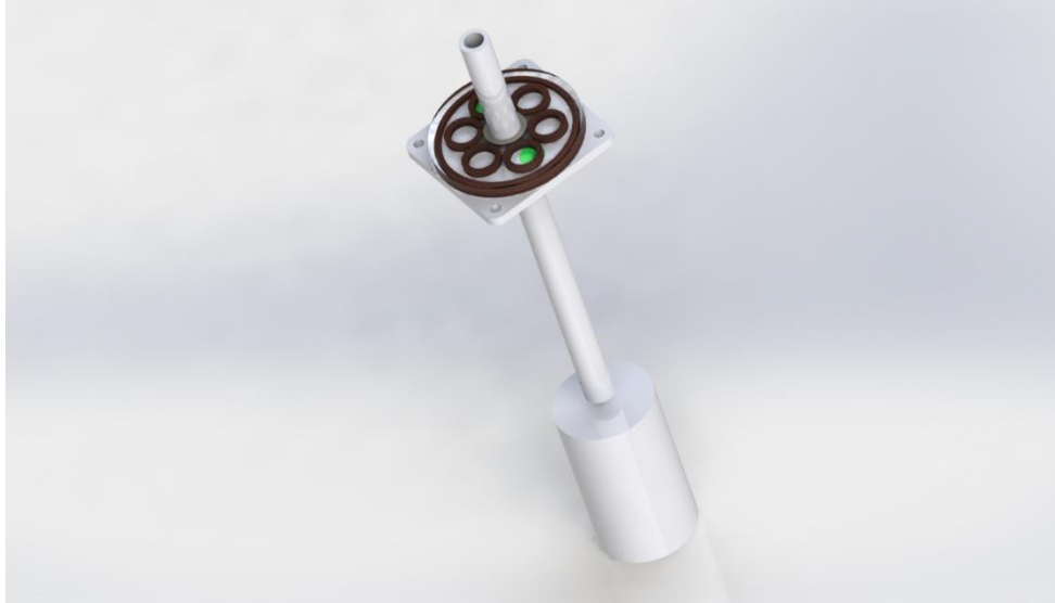
Figure 6: Single Magnet Disk Generator Final Version.
