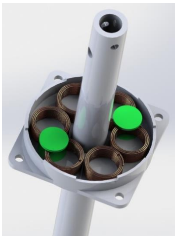
Figure 7: Dual Magnet Disk Without Cover Top.
