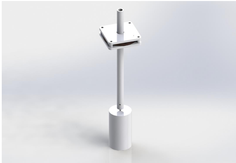
Figure 9: Dual Magnet Disk Generator/Rotary Transformer Final Version.
