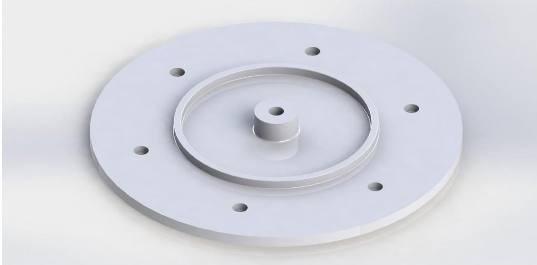
Figure 12: Bottom Cast Form Plate, Final Version. With Fillet On Axel Replacement Cylinder And Increased Width Of Plate.
