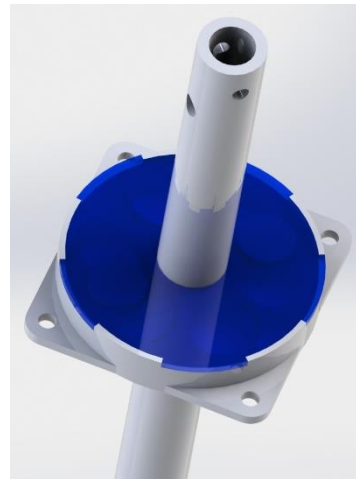
Figure 8: Dual Magnet Generator Housing.
