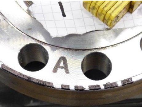
Figure 60 - Environmental seal after 0 rotations.
