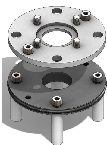
Figure 16 - Separation of motor flange and gear cover.
