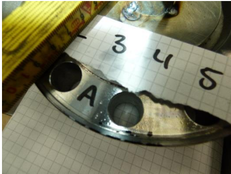
Figure 62 – Environmental seal after 30 rotations. Marks are still clear on the outer edge.
