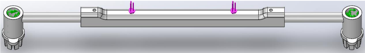
Figure 52 - Forces and fixtures on mounting dolly.
