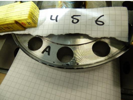
Figure 63 – Environmental seal after 40 rotations. No difference from Figure 62
