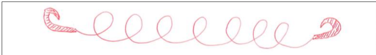
FIGURE 23: A tension spring mounted by hand or with the use of pliers
