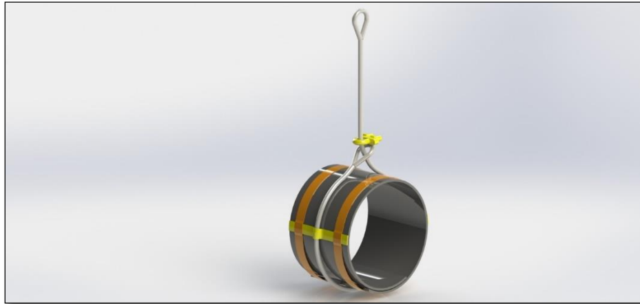
FIGURE 13: A double choke hitch
