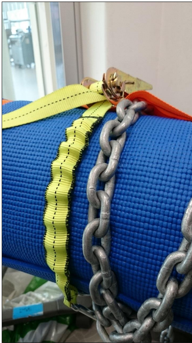
FIGURE 84: Elastic straps on the tightening mechanism
