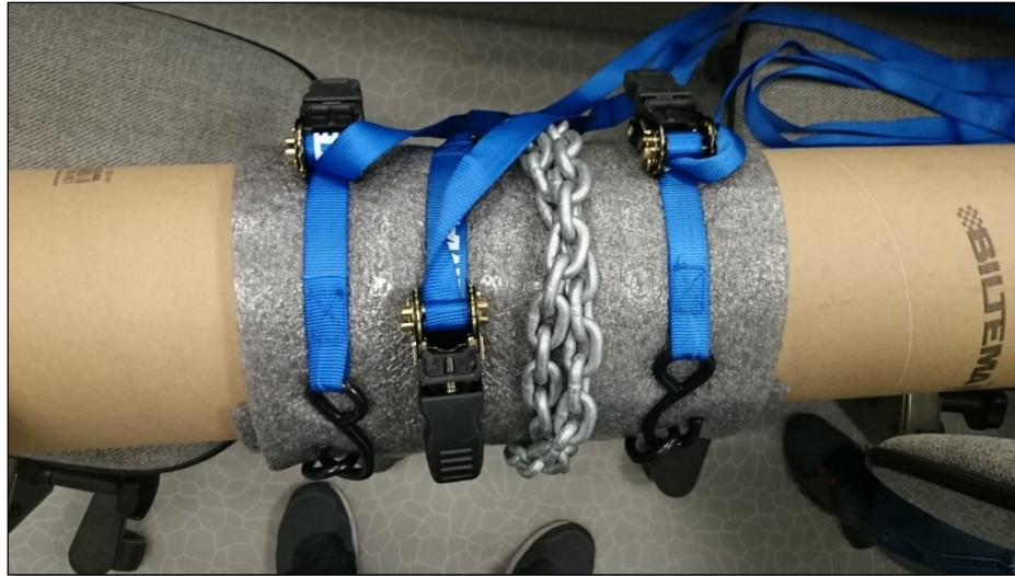
FIGURE 82: Ratchet tie-down used as tightening mechanism for the chain
