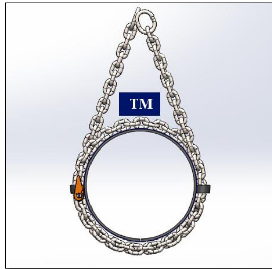
FIGURE 45: The placement of the tightening mechanism on the pipe
