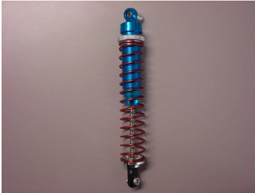
Figur 1: 110mm aluminiums demper
