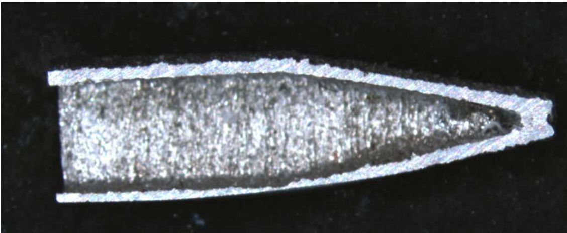
Figure 24 Cross section of a capsule used in generation three device, note the inner surface roughness.
