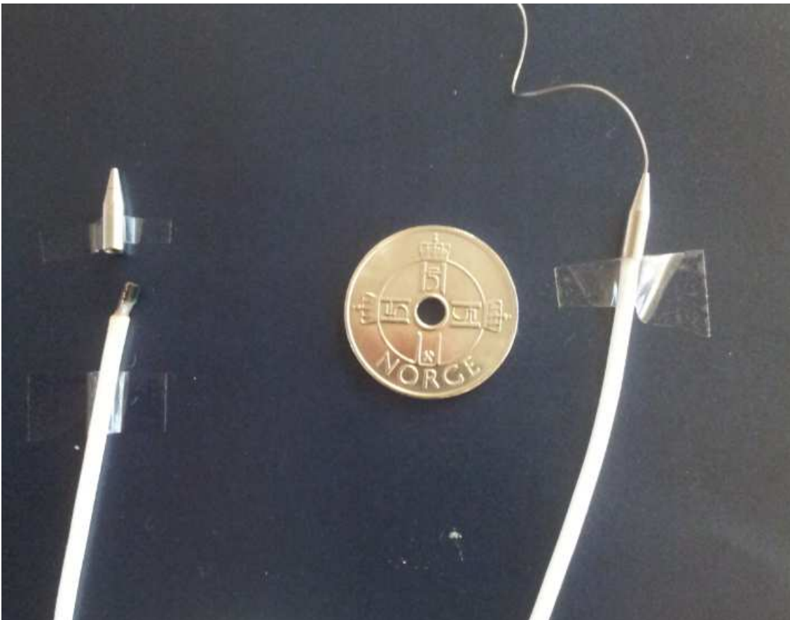
Figure 19 Left, a capsule and a sensor-cable assembly prior to potting, right, an assembled device. Coin shown for scale purposes.
