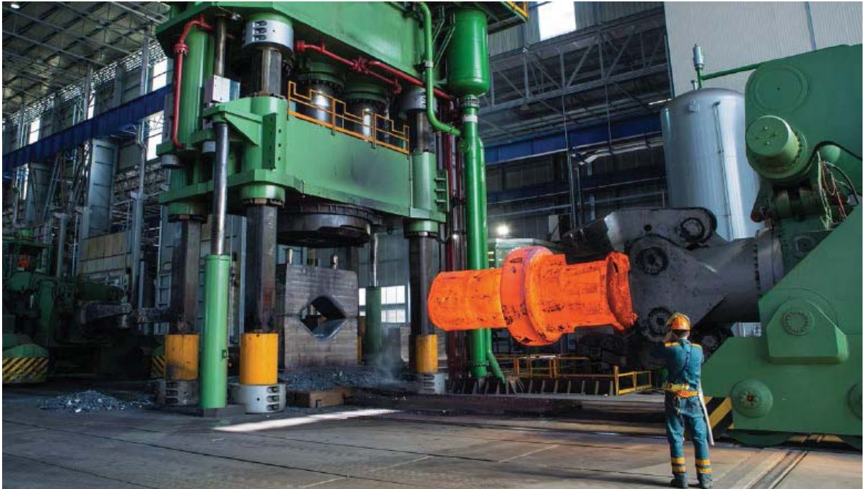
Figure 11, Forge and manipulator with workpiece
