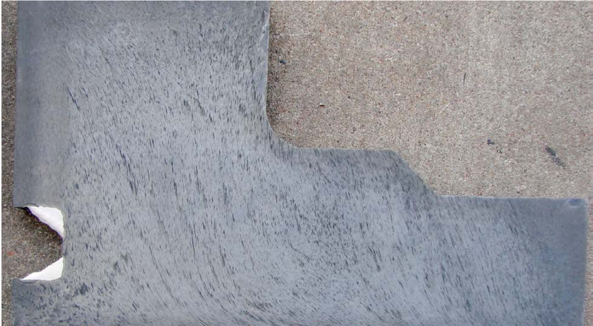
Figure 8, Grain flow of forged flange
