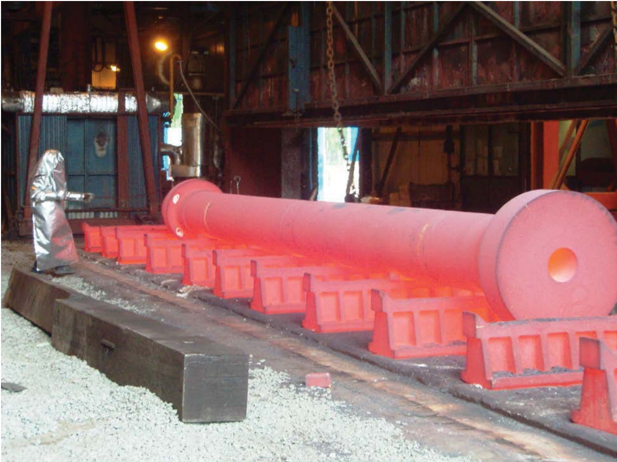
Figure 7, Part ready for quenching
