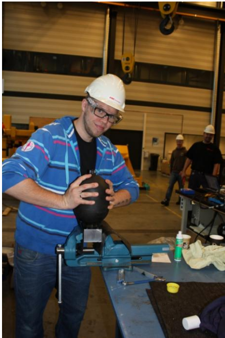
Figure 5: Mounting the accumulator to the adapter
