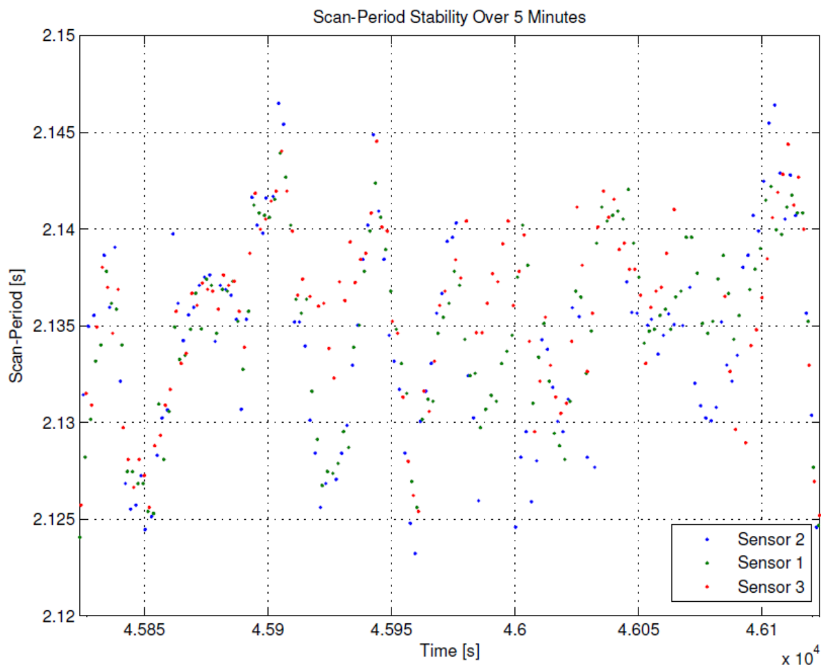
Figure 19. Correlation diagram over 5 minutes (counting seconds from 00:00 am on recording day). The scatter diagram illustrates correlation for scan-period as determined by Sensor 1, Sensor 2 and Sensor 3. Time between grid lines on the time axis is 50 seconds. Over 50 seconds scan-periods for 23 mainlobes per sensor are detected. Averaging over 5 mainlobes, corresponding to about 11 seconds, seems appropriate.
