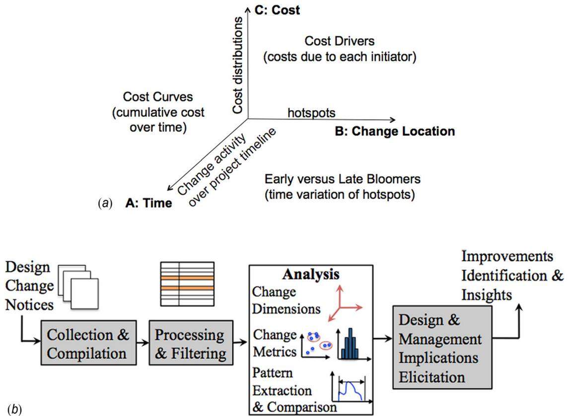
Fig. 1.4 (a) Dimensions of engineering change and (b) engineering design change analysis process
