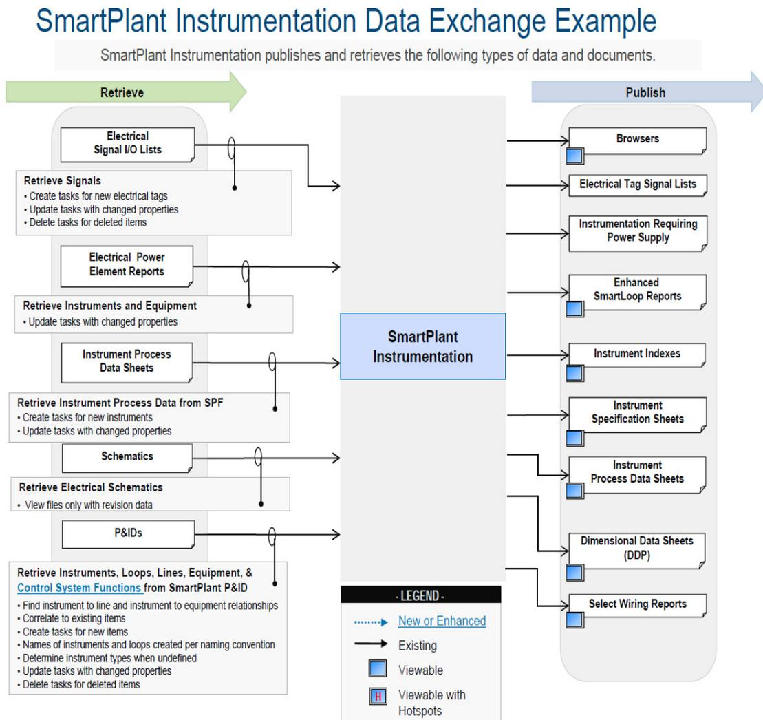
Fig. 4.10 SmartPlant Instrumentation Data exchange [35]
