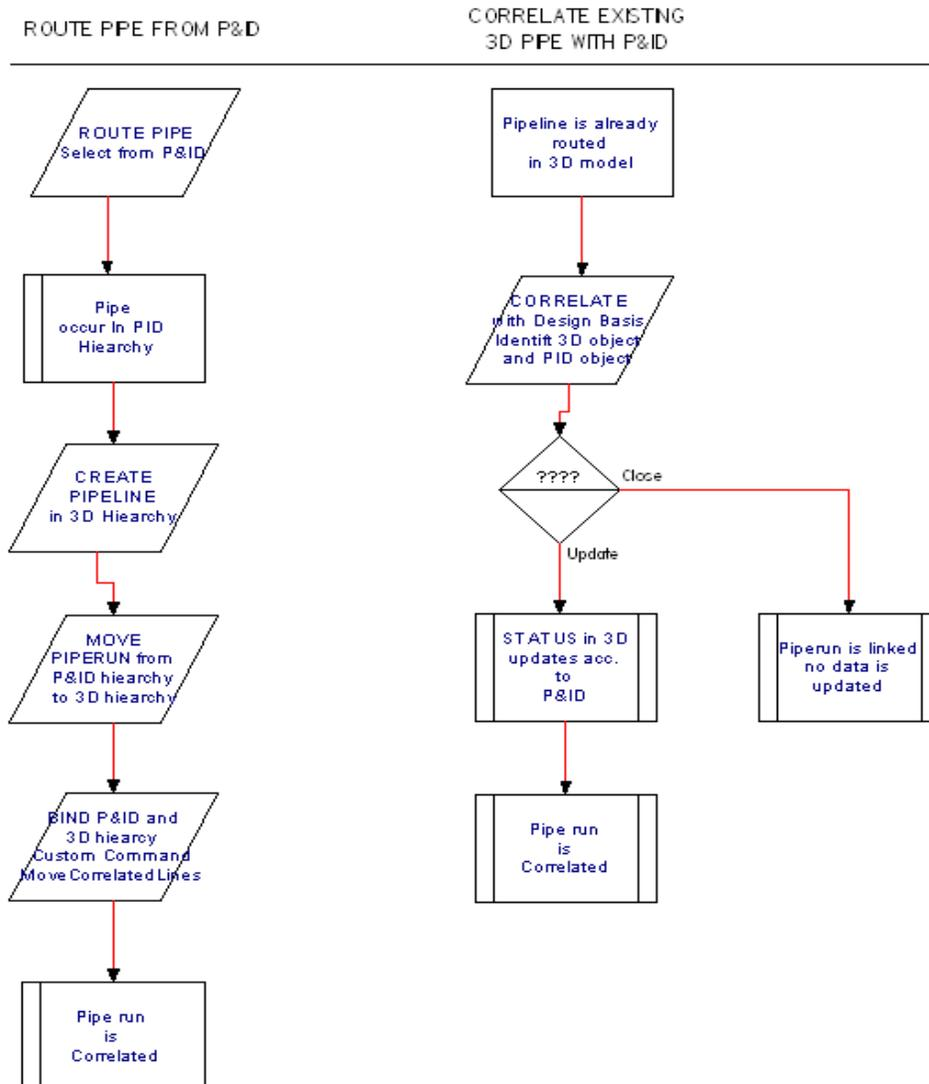
Fig. 4.3 Example of Integration checking for the Process P&ID
