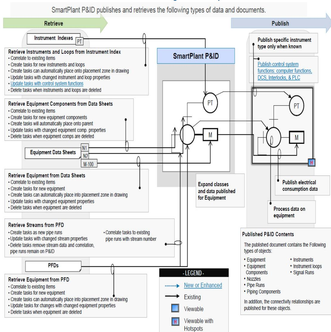
Fig. 4.11 SmartPlant Process & Instrument Diagram (P&ID) exchange [35]
