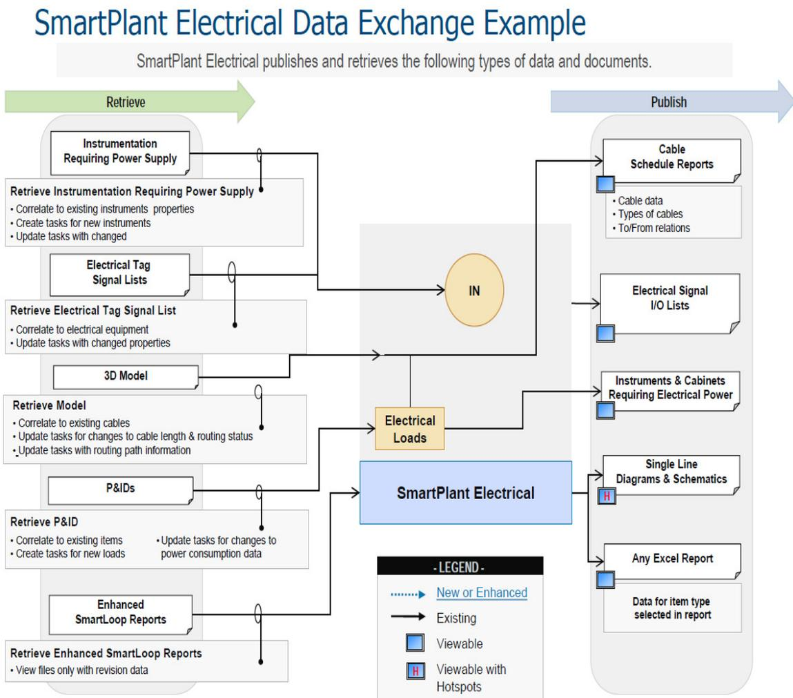
Fig. 4.9 SmartPlant Electrical Data exchange [35]
