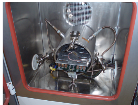
(b) Pressure chamber inside temperature chamber.
