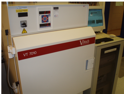
(a) Temperature chamber and control equipment.
