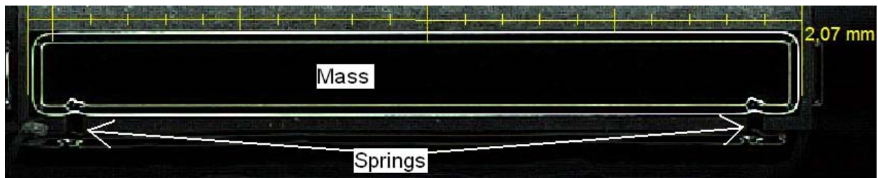
Figure 7-26: Craig-design accelerometer structure.
