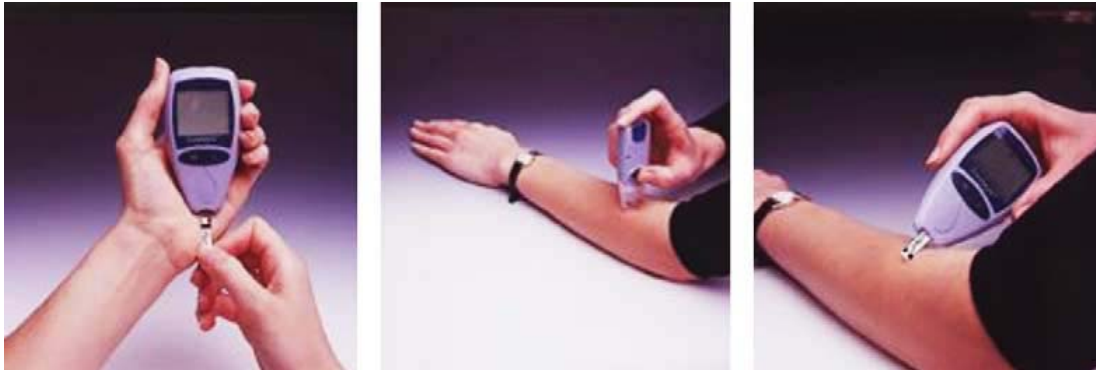
Figure 3 Measurement of the blood glucose level by external sampling requires three steps: (i) Insert the sensor test strip in the reader; (ii) Puncture the skin by a lancet; (iii) Sample the blood drop. Figure from Newman and Turner [28].
