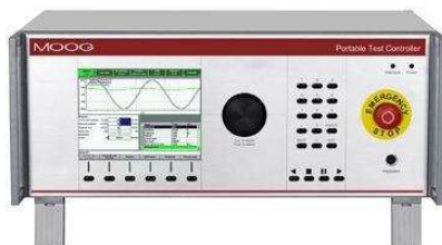
Figure 21: Standalone Portable test controller
