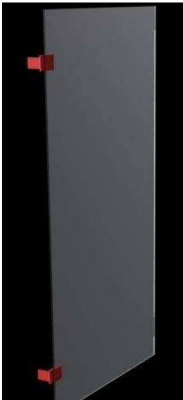
Figure 103: Hinged protection plates
