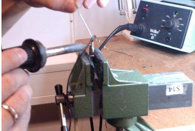
Picture 3: Soldered cable
