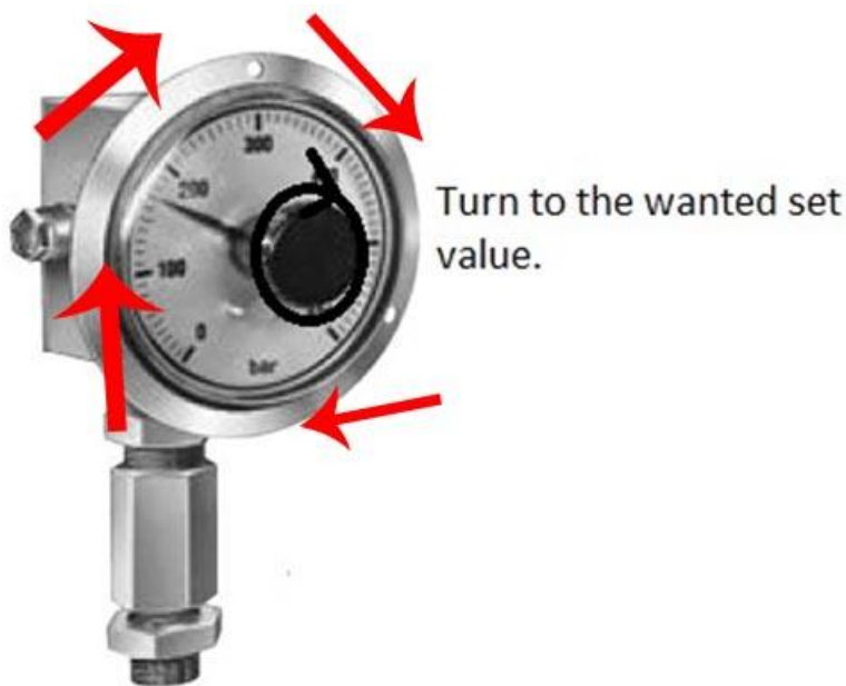
Figure 7: How to set the pressure switch
