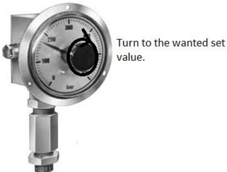
Figure 4: Where to set the wanted test pressure
