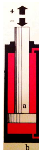
Figure 29: Inside of a single rod cylinder
