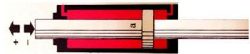
Figure 59: Function of cylinder with double rod. [16]
