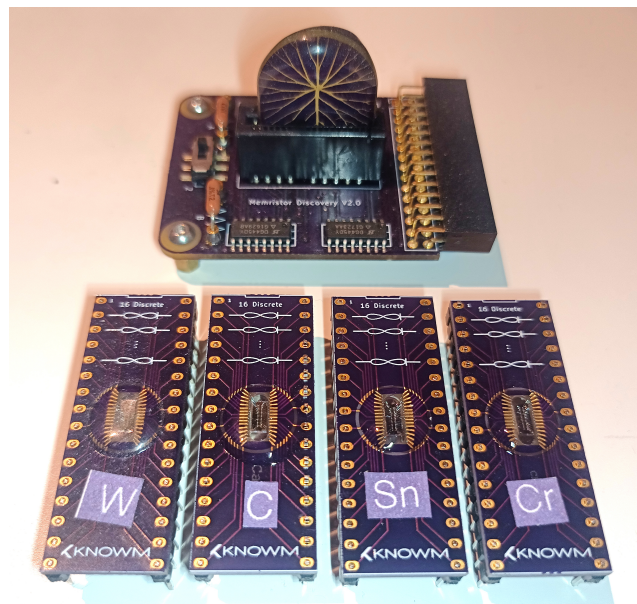
Figure G.6: Overview of used memristors. Shown are four different SDC models (W is Tungsten, C is carbon, Sn is Tin, Cr is Chromium with different characteristics in two different packages. See Knowm datasheet [238].
