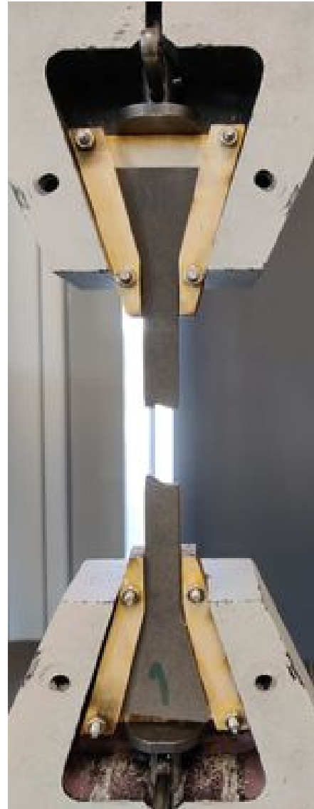
(b) The test specimen N0_1 after executed test.
