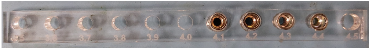
(b) Inserts soldered into test strip.
