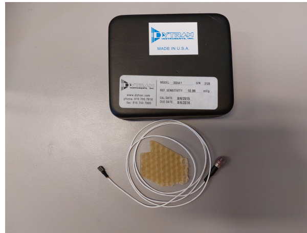
Figure 9.32: Dytran DY 3224A1 accelerometer
