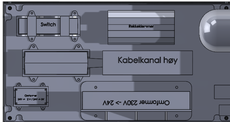
Figure 9.25: CAD-model of Power Supply seen from above.
