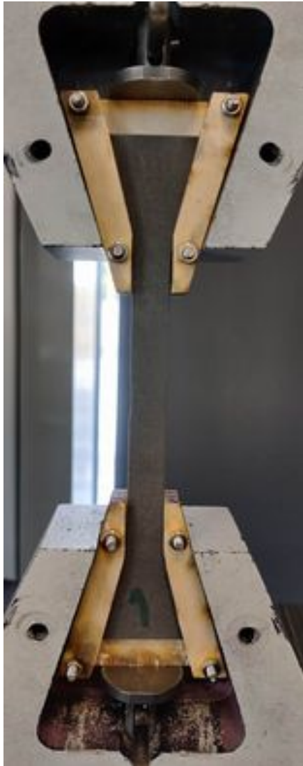
(a) The test specimen N0_1 placed in the tension test machine.
