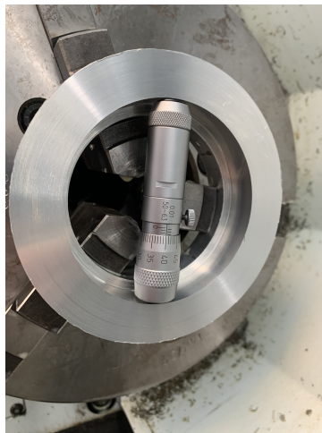
Figure 10.13: Measuring bearing clearance
